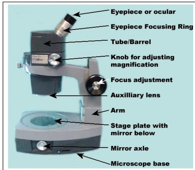
**Figure 5.** Parts of a Stereomicroscope (aka dissecting microscopes)
