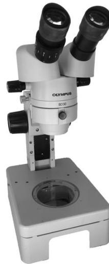
**Figure 2.** Dissecting microscope
