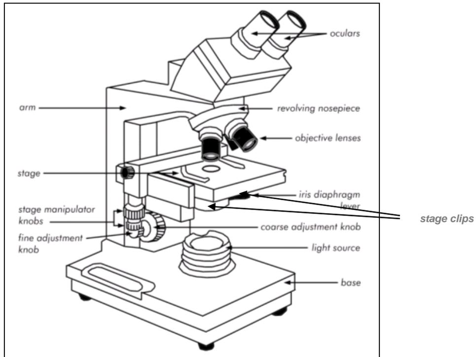
**Figure 3:** The binocular compound light microscope.
