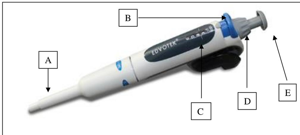
1. Adjust the dial (D) on the pipette so that the numbers (C) indicate the volume you wish to dispense. The volume that can be dispensed by our devices is measured in microliters ( $\mu\text{l}$ ).
