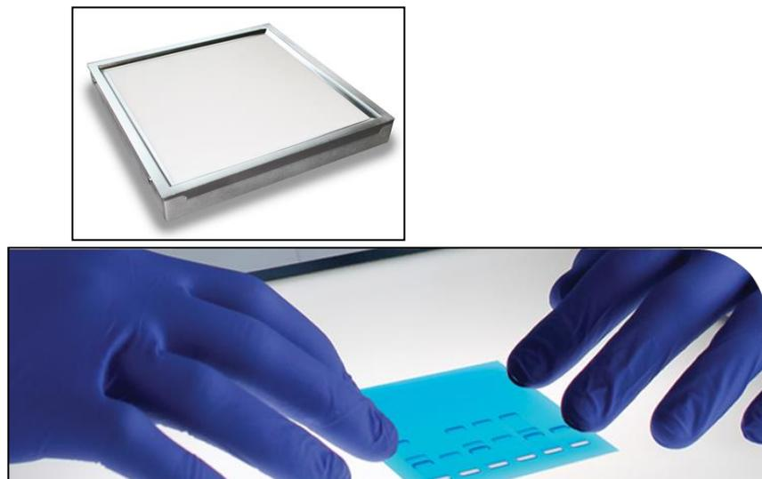
**Fig. 8.** White light box (left) and visualization of DNA bands on gels.
