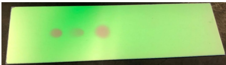
Figure 4. Example of a TLC plate under UV light, showing the presence of eluted spots
