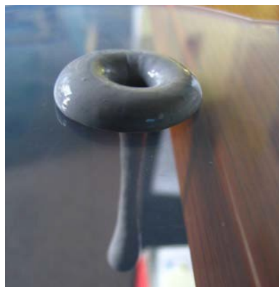
Figure 11.17. Picture of silly putty's non-Newtonian flow [https://upload.wikimedia.org/wikipedia/commons/f/f3/Silly_putty_dripping.jpg]
