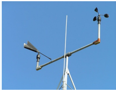
Figure 6.3.4: Anemometer (right) and Wind Vane (left) (Courtesy NOAA, Source)
