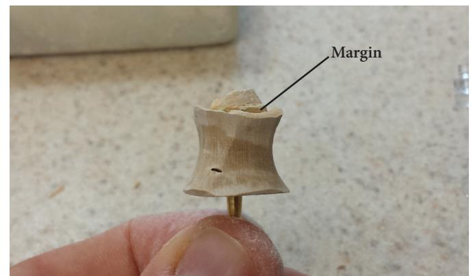
Figure 8. Die after grinding
